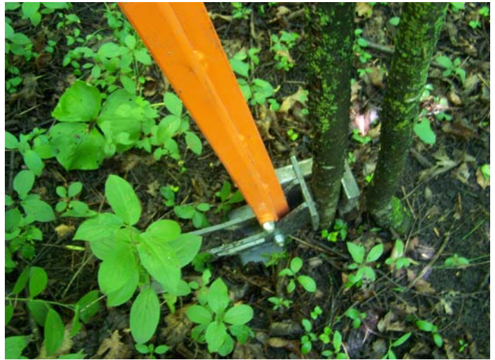
The Extractigator™ gripping on to a European Buckthorn tree. Photo by Carly Dow, MNS
